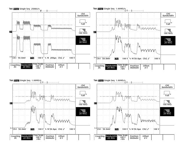
Time base - 50us/200us Chl - 50A/div; (measured with 0.001R non-inductive shunt) Lamp current - 0 to 150A Ch2 - 100V/div Lamp voltage - 0 to 400V
